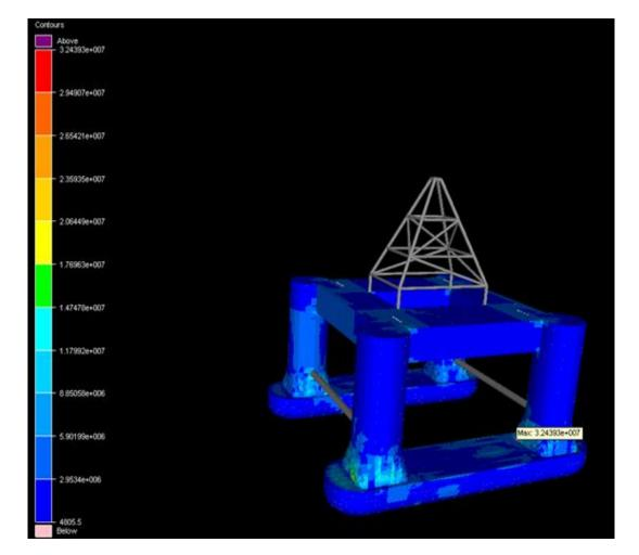
Critical Location: Pontoon-column connection (Max.Von-Mises Stress)
